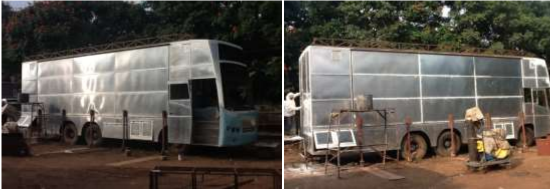
Figure 2 Five landing wheels which were assembled/attached to the outside body of expandable portion before the expansion
