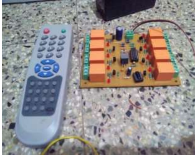
Fig: Transmitter and receiver of IR remote control
