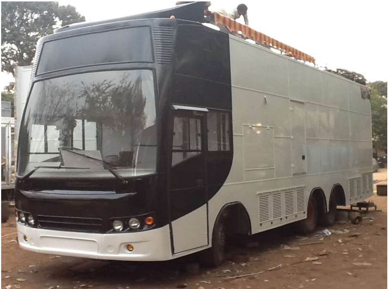
Final Stage of Fabrication of Expandable Auditorium on Wheels built on Truck Chassis
