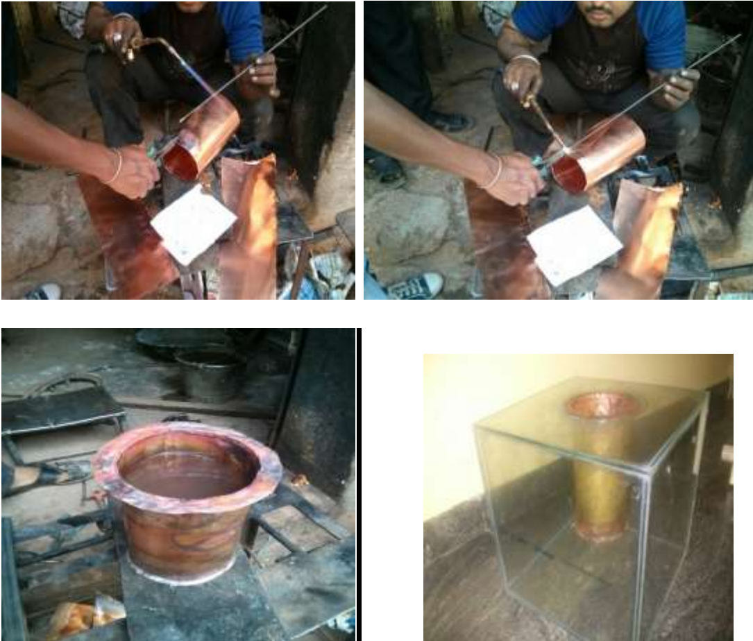
Fig : Fabrication Process
